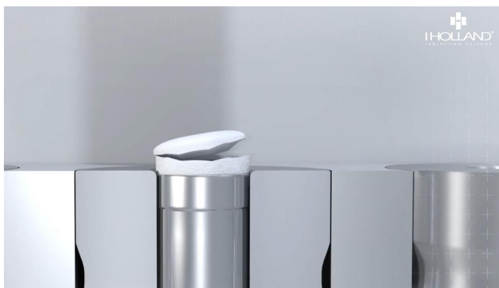
Figure 4: A typical example of capping
