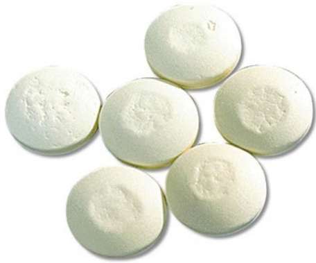
Photo 2: Core erosion is a common defect for tablets with very round profiles, especially when put under strain during coating. The tooling should be redesigned with a less concave profile to help the tablets withstand the coating process.
